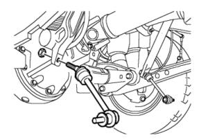
5. Install the new anti-roll bar links into the long arm / anti-roll bar.
